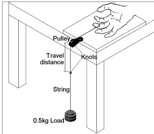
Fig. 2: Schematic view of the experimental setup
